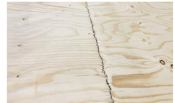
The bottom side veneer joint is also visible and the resorcinol glue line is visible.
