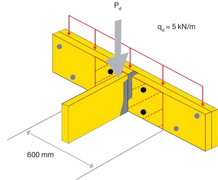
The values given in this table are maximum medium term design side loads meeting the capacities of the fixing details. The Engineer should also check that all other strength and stiffness design criteria are met (e.g. moment, shear, bearing and deflection). The values given in this table include any design UDL load adjacent to, and supported by, the fixings. The design UDL must be subtracted from the table value in order to determine the maximum point load, for example:
